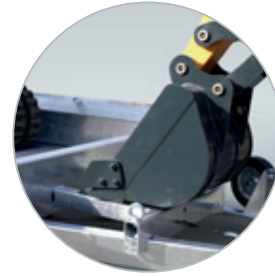
Standard equipped with excavator bucket support on the A-frame
