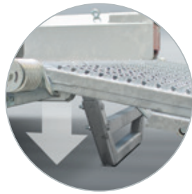
Integrated propstands on tailgate ramp
