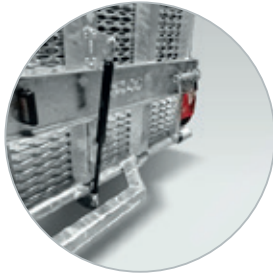
Accessorie: Gas spring for tail ramp (ramp heigth 150 cm)
