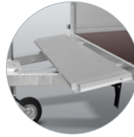
Front-panel can rest on the A-frame
